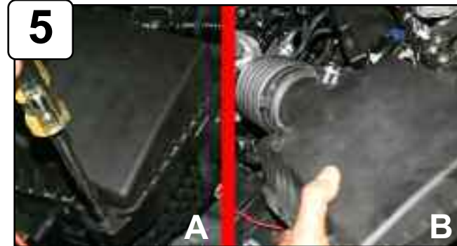
With 8mm socket or wrench loosen the 4 screws holding in upper half of air box and remove.
