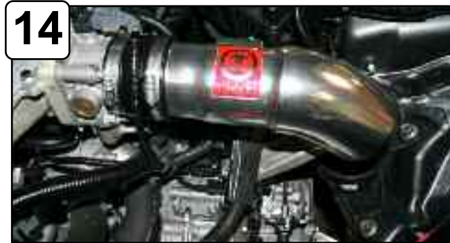
14 3.5L engine , install tube with 05-01028 coupling and two #48 clamps. Do not tighten.
