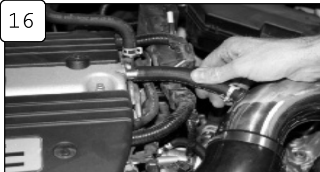
Install provided 5/8" hose to engine and tube. Re-connect MAF sensor harness and battery terminals.
