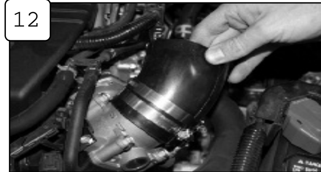
Install elbow coupler to throttle body and position using clamps provided. Do not tighten.
