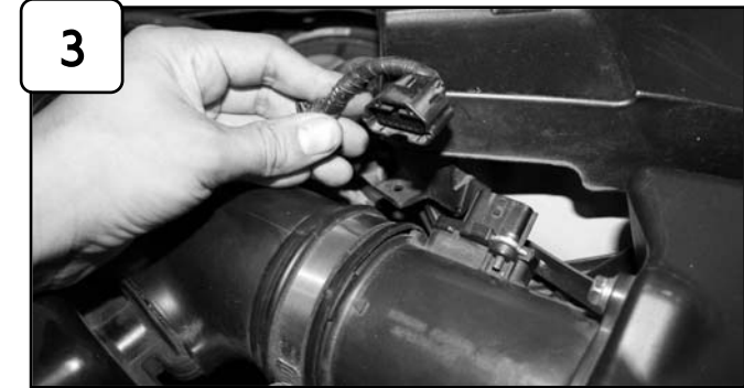
3 Disconnect MAF sensor harness. Unclip upper half of air box. Loosen clamps using 10mm socket or wrench.
