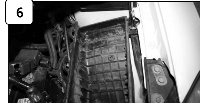
6 With 10mm socket or wrench loosen bolt securing in bottom half of air box and remove.
