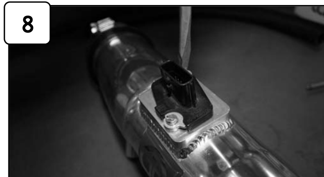
8 Install MAF sensor to upper tube assembly and secure using provided M4 screws.
