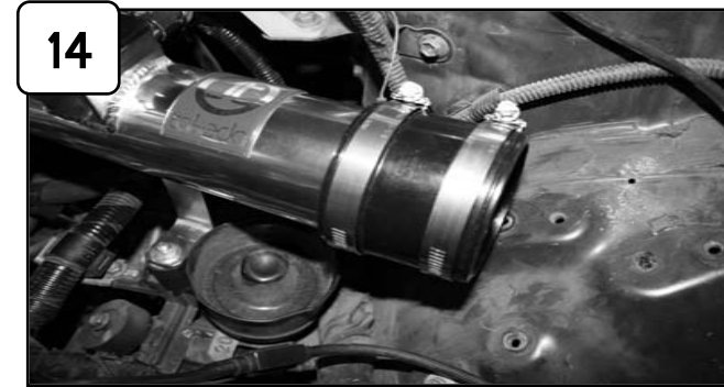
14 Attach 05-00418 coupling with clamps to upper intake tube assembly. Do not tighten.
