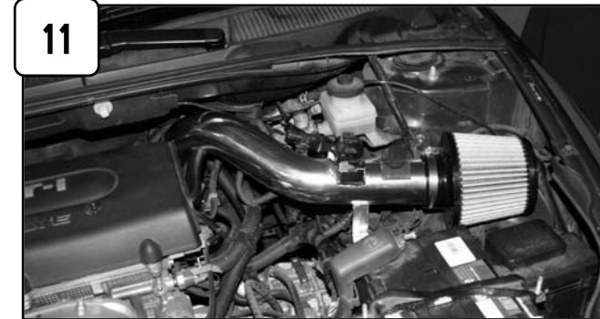
11 Install air filter and tighten using 5/16" nut driver. Tighten all clamps using 5/16" nut driver. Attach pre filter to filter if desired. Your short ram intake is now complete.
