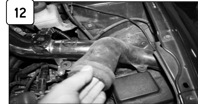
12 Remove air filter and factory snorkel plastic unit.
