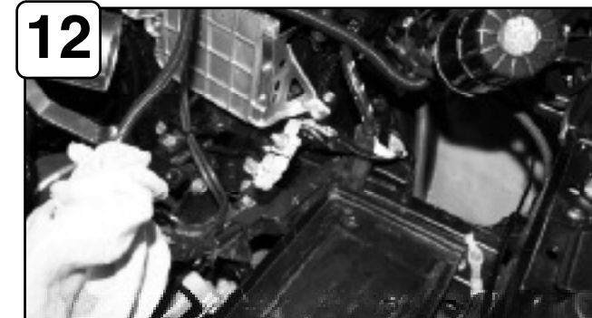
12 Remove air filter. Loosen battery bracket with 10mm socket or wrench and remove battery. Remove factory snorkel plastic unit. Cover positive terminal with rag or towel.
