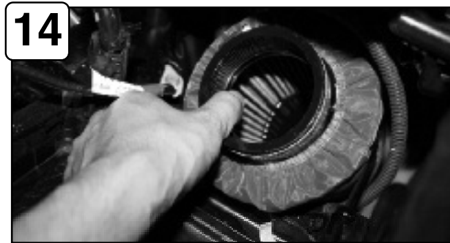
14 Attach pre filter (if not already done) to filter and place filter inside front of driver side wheel.
