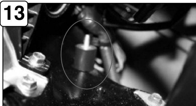
13 Install and tighten isolation mount to frame.
