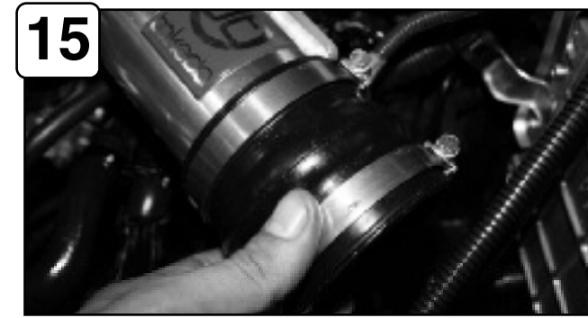
15 Attach hump coupler with clamps to upper intake tube assembly. Do not tighten.
