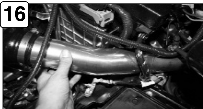
16 Install lower intake tube to hump coupler and isolation mount.
