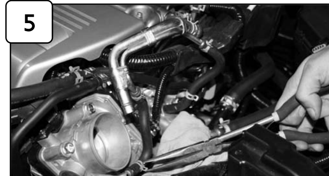
5 Remove crank case line attached with throttle body coolant line. Have a shop towel or rag handy to catch any leaking coolant. Use pliers to remove both lines. Save small clamps for later install. Caution: Coolant may leak from line when removing!
