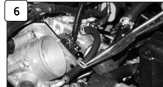
6 Replace throttle body coolant line with 5/16" hose provided and secure with clamps used from step 5.
