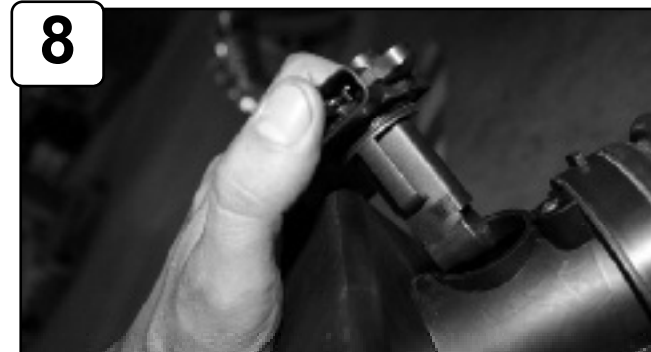
With phillips screwdriver, loosen and remove MAF sensor from stock air box.
