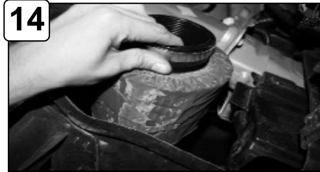
13 Install reducer coupling with clamps to turbo housing. Tighten clamp on housing only.
