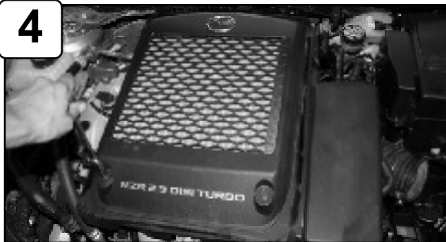
With 10mm socket or wrench loosen the 2 bolts holding in engine cover and remove.
