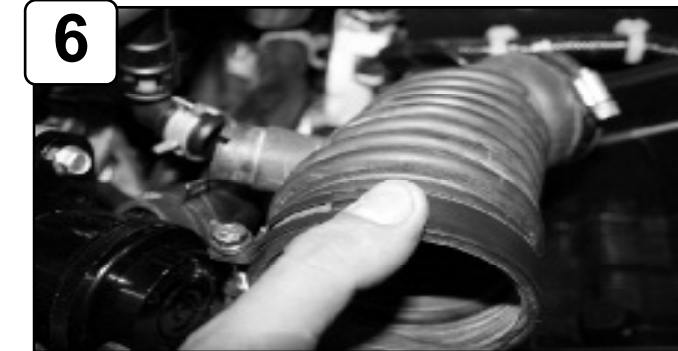
Disconnect crank case line using pliers. Remove stock intake tube.
