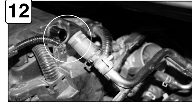
12 With pliers, remove the pressure clamp holding the crank case breather line to the valve cover and pull it off.
