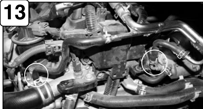
13 When the engine has cooled completely, remove the radiator cap to relieve pressure then with pliers remove both pressure clamps securing the stock coolant line to the engine (circled in white). Make sure to have a rag handy to catch the small amount of coolant left in the line.
