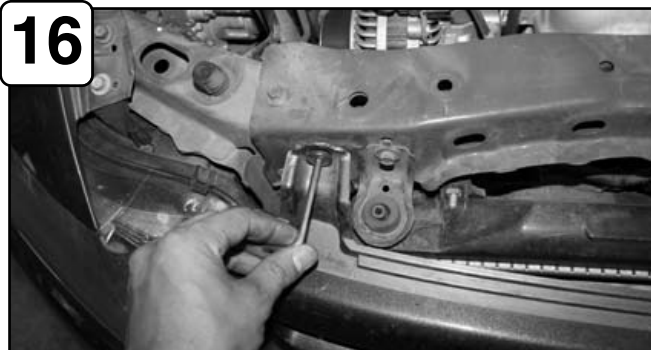
16 Remove both bolts holding the top of the bumper to the radiator support. (Passenger side and driver side)
