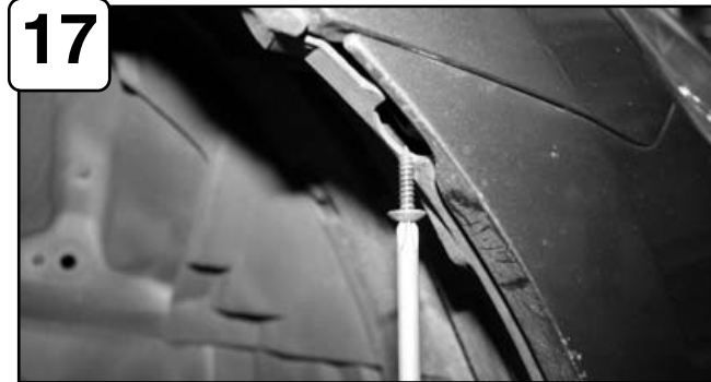
17 Remove both screws holding the bumper to the fenders. (Passenger and driver side)
