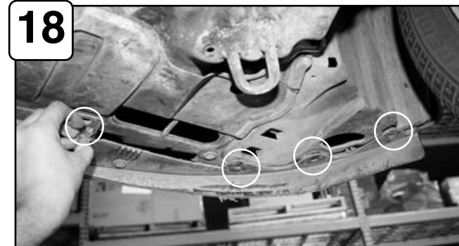
18 From underneath the vehicle, remove all the push clips holding the lower portion of the bumper to the splash shields.
