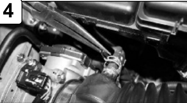
Loosen clamp on throttle body using 10mm socket or wrench. With pliers pull crank case line away from tube.
