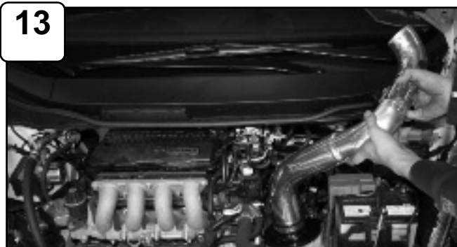
13 Install intake into vehicle.
