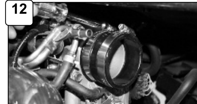
12 Install straight coupler to throttle body and position using clamps provided. Do not tighten.
