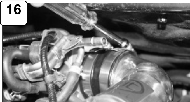
16 Tighten all clamps using 5/16" nut driver.
