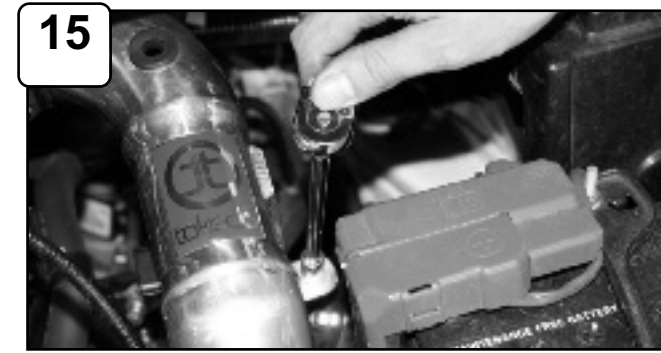
15 Tighten down intake using provided flat washer, wavy washer and hex screw.
