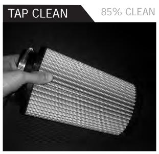
You can tap your Pro Dry S filter and return it to 85% of its original airflow. Simply remove the filter from the intake kit and lightly tap it on a solid surface. Tap and turn the top and bottom of the filter until most of the visible dirt has been released. Reinstall the filter in your vehicle. Do not apply oil to the filter.
