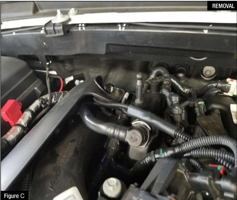
Refer to Figure Cfor Step 3.Step 3: Remove large engine cover on top of engine. Loosen small plastic cover on left side of engine bay.
