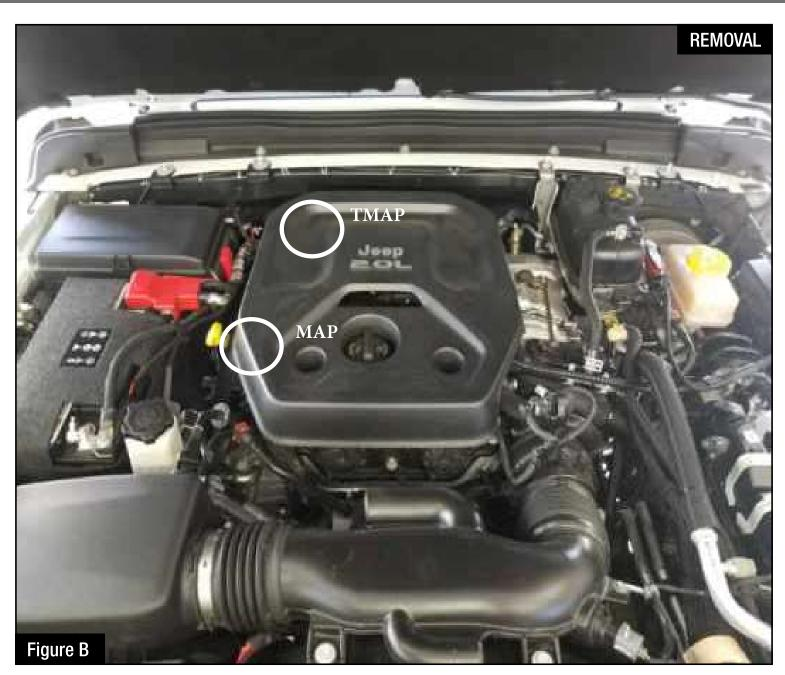
Refer to Figure B for Step 2. Step 2: Locate the TMAP and MAP sensor. The TMAP Sensor is located on the charge pipe on the left side of the engine bay(circled above). The MAP sensor is on top of the intake manifold, next to the oil dipstick (circled above).
