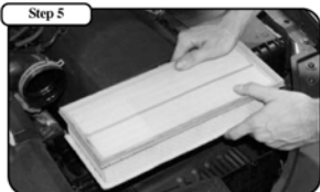
Remove the stock air filter and plastic grill from the factory air box.
