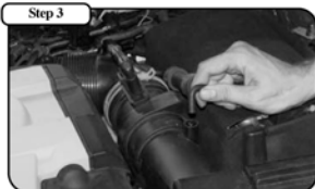
Disconnect the MAF sensor and unplug the breather tube that are located on the top side of the stock intake tube.
