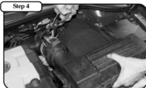
With a pair of pliers, loosen the clamp holding the MAF sensor to the stock intake tube and remove the cover and sensor from the vehicle.
