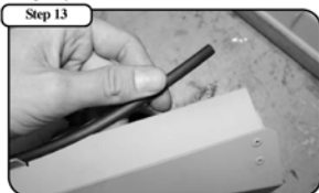
Place trim seal on the bottom side of the intake cover.
