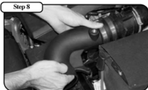
Insert the aFe intake tube along with the coupling and clamps onto the MAF sensor. Secure the intake tube using the provided screws.
