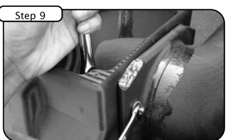
Install tube to outside of housing. Tighten using screws, washers and nuts provided with 7/16" socket or wrench.
