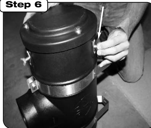
Line up cover clips to Dzus fasteners and secure cover.
