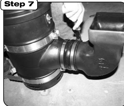
Install your snorkel with hump coupler and clamps and tighten. (Snorkel and band clamps can be adjusted)
