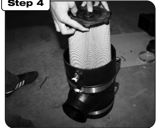
Install filter into canister and tighten using 5/16" nut driver. (Use cut out slots to tighten.)
