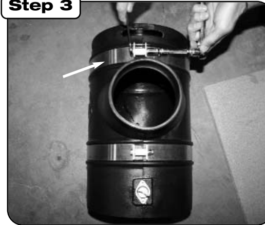
With 10mm socket or wrench, tighten down band clamps with hardware provided. Use 1 flat, 1 lock washer per screw (Make sure nylon spacer is between clamp to keep from collapsing.)
