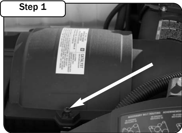
Loosen the phillips screw on the air box and remove the cover to access the air filter.
