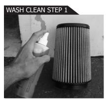
You can wash your Pro Dry S filter and return it to 100% of its original airflow. Remove the filter from the intake kit and simply spray the filter with .aFe cleaner and let sit for 10 minutes.
