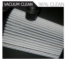
You can vacuum your Pro Dry S filter and return it to 96% of its original airflow. Remove the filter from the intake kit and vacuum away the dirt using a shop vacuum or regular house vacuum. Reinstall the filter in your vehicle. Do not apply oil to the filter.
