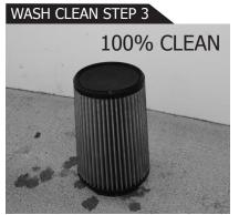
Allow the filter to dry completely (our synthetic media dries quickly and should dry within a few hours in normal conditions). Reinstall the filter in your vehicle. Do not apply oil to the filter.
