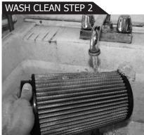
Rinse the filter with clean water to remove the dirt and excess cleaner. Continue rinsing until the water runs clear.
