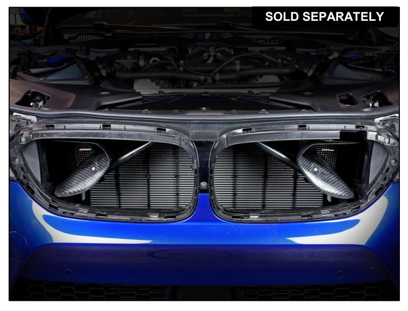
If you have also purschased the aFe POWER Carbon Fiber dynamic Air Scoops (P/N: 58-10005SC), follow the install instruction provided with the scoops to install them behind the grilles and guide the extra air flow to the air intake system.
