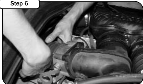
Step 6 Install the smaller 3" coupler and clamps on the throttle body. Do not tighten clamps at this time.
