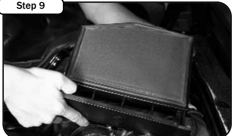
Step 9 Open the air filter access tray on the side of the air box and remove the OE air filter.
