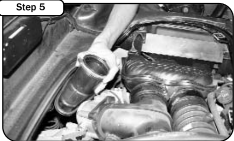
Step 5 Carefully remove intake tube out of the engine compartment.
