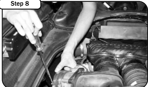
Step 8 Carefully install the new intake tube in the engine compartment. Tighten all four clamps securing intake tube.
