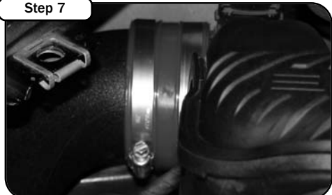
Step 7 Install the larger 3.25" coupler and clamps on the air box. Do not tighten clamps at this time.
