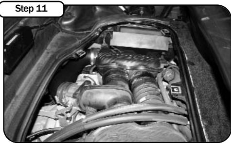
Step 11 Your installation is now complete. Make sure you tighten all clamps and check all electrical connections. Re check periodically
