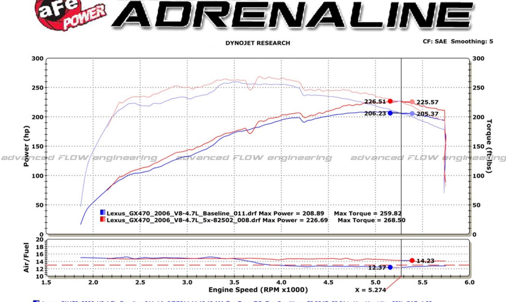
Lexus\_GX470\_2006\_V8-4.7L\_Baseline\_011.drf - 3/7/2014 11:46:18 AM Run Type: RO Run Conditions: 78.36 °F, 29.01 in-Hg, Humidity: 26%, SAE: 1.02 OE AIS, OE Exh, 3rd Gear Run, 10% Brake before run, (RPM pick up on first cylinder driver side closer to fan. (SportMode)(Height Control Off) Official Run.
