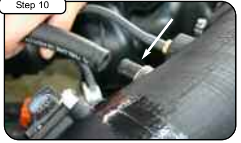
Connect 1/2" hose to new tube and tighten clamp with flat-head screwdriver. Re-connect MAF sensor harness and fuel regulator.
