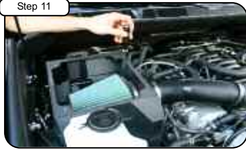
Place air filter into housing and tighten using 5/16" nut driver.
