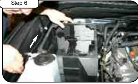
Install trim seal provided to auxiliary on side. Install filter adaptor to new housing with button head screws provided and secure. Install new housing using screws and grommets from step 5.
