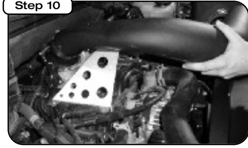
Step 10 Place coupler (05-00464) on the throttle body (see diagram below for correct coupler position) and the housing. Position intake duct into engine bay and tighten down the clamps.
