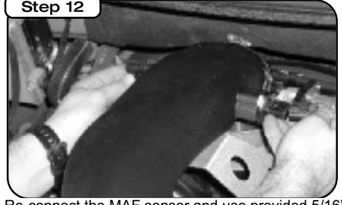
Step 12 Re-connect the MAF sensor and use provided 5/16" breather hose to connect the intake duct to the crankcase breather on the engine valve cover.
