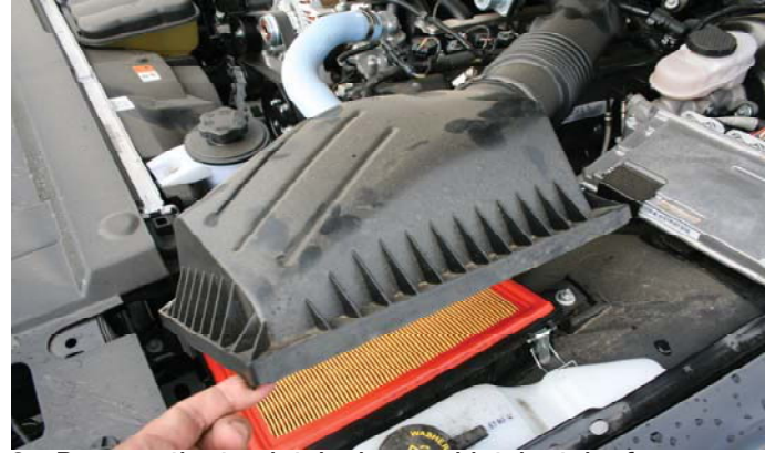
6- Remove the top intake box and intake tube from vehicle and put it aside.
