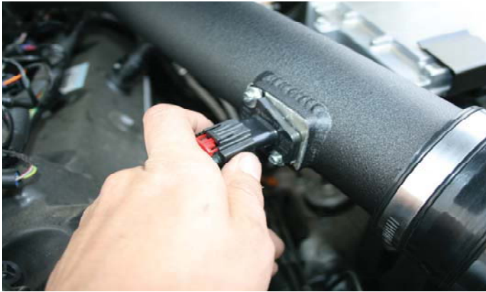
18- Reconnect the MAF sensor onto the intake tube and lock the plug by pushing in on the red safety lock.
