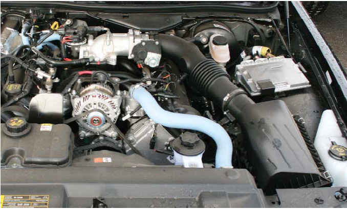
1- View of stock intake system.
