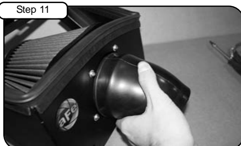
Attach the coupler with the clamps provided to the filter adaptor. Do not tighten clamps.
