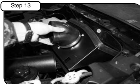
Install the new housing into vehicle. Engage the clips, secure housing and connect the intake tube to coupler.
