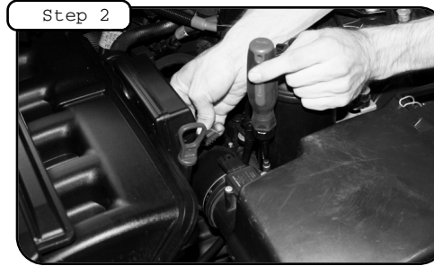
Disconnect MAF sensor. Loosen clamp on air box. Unclip upper half of airbox to remove lid and disconnect MAF sensor harness.
