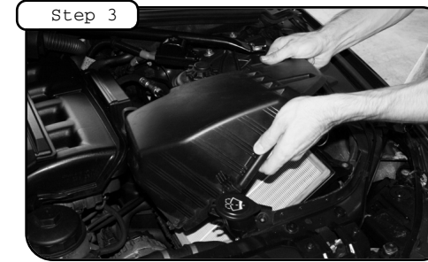
Loosen bolt with 10mm socket or wrench and save for later use.
