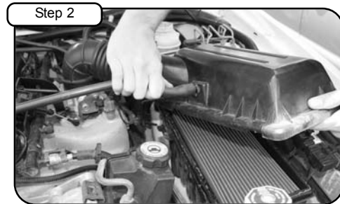
Step 2 Unclip upper half of air box and pull back crankcase line.
