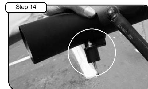
Step 14 Install isolation mount to bracket with flat/wavy washers and nut provided. Do not tighten.
