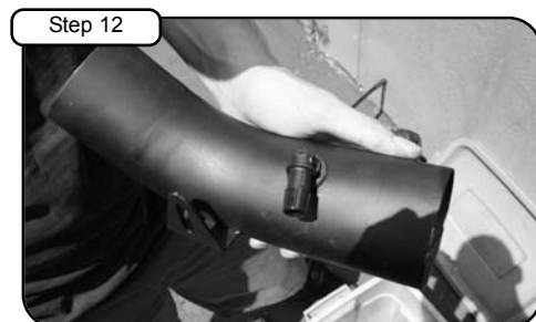
Step 12 Install 1/2" fitting in grommet.
