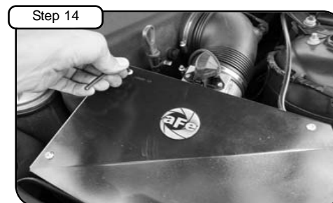
Step 14 Install cover using button head screws provided and tighten using 5/32" allen key. Re-connect MAF sensor harness.
