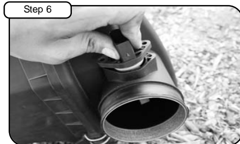
Step 6 Remove MAF sensor from stock air box using T20 torx bit.
