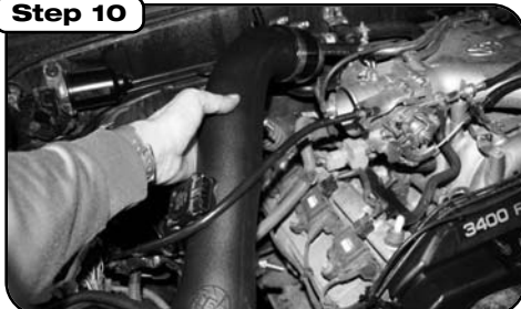
Step 10 Install throttle body coupler to intake tube and using provided hose clamps and install intake tube. Use rubber isolation mount between tube bracket and heat shield.
