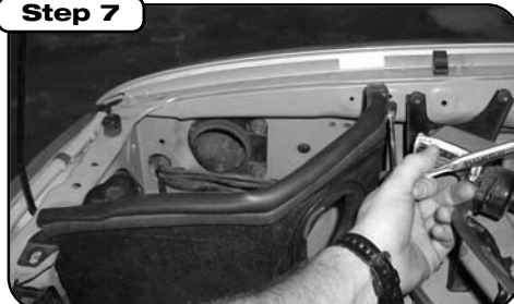
Step 7 Install heat shield using provided hardware and reconnect ground wire to fender if applicable. Install 7/16" trim seal to top of housing.
