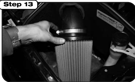
Step 13 Install filter to intake tube. Re-position clamp and tighten. Do not use oil or grease. Reconnect factory harness to MAF Sensor
