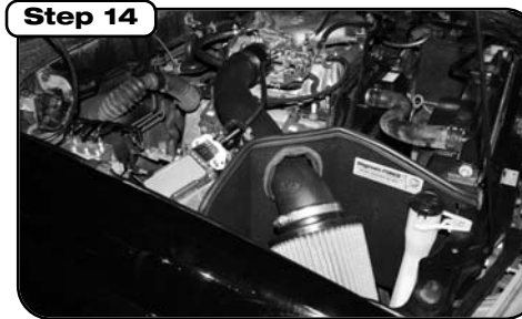
Step 14 Make sure all hoses and clamps are tight and that all electrical components are secure. Check and re-tighten connections and filter after a few hours of operation. Thank you for choosing aFe!
