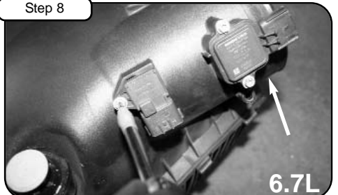
(6.7L remove and install temp sensor, see step 7 ) . 6.7L, remove MAF sensor and install to new tube with screws and gasket (Make sure gasket is between sensor and tube) Install grommet only to tube. The 6.7L will not use small phillips screws.
