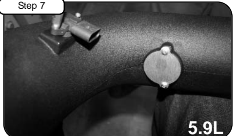
With T-20 torx bit remove temp sensor and (with gasket and screws provided) install into new tube. (5.9L place MAF cover with gasket and tighten using short screws provided.) Install plug into the hole in tube for crank case line.
