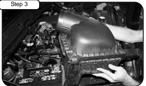
Disconnect air temp sensor. ( 6.7L, disconnect MAF sensor ). Lift up and pull OE air box out of vehicle.
