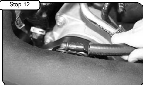
Step 12 Install new 3/8" hose provided to valve cover side and new tube side.
