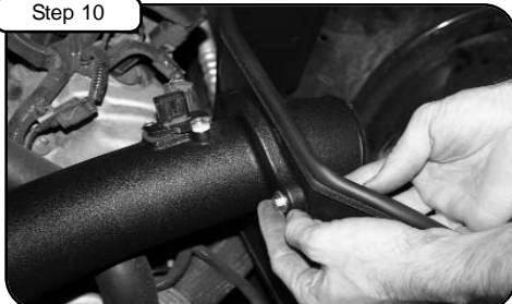
Step 10 Install screws/nuts and washer provided to mount tube to housing. Tighten using 10mm socket or wrench.
