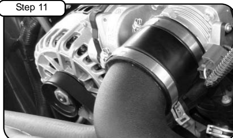
Step 11 Tighten clamps with 5/16" nut driver.
