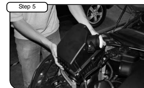
Step 5 Remove air box from vehicle.
