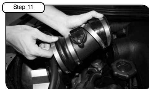
Step 11 With couplers and clamps provided, install tube into vehicle.
