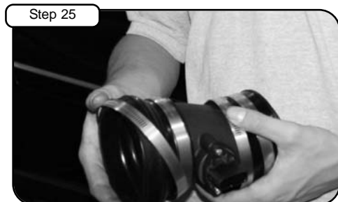
Step 25 With couplers and clamps provided, install tube into vehicle.
