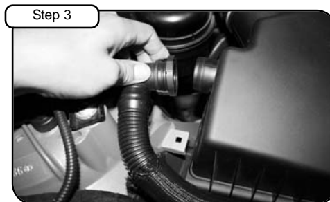
Step 3 Disconnect smog line from air box.
