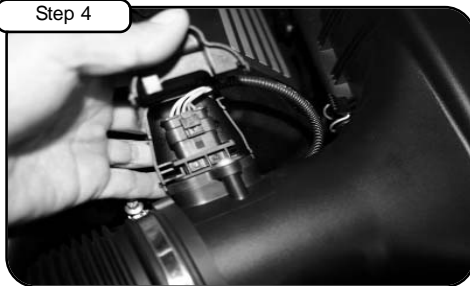
Remove the MAF sensor cover. Disconnect the MAF harness from sensor.
