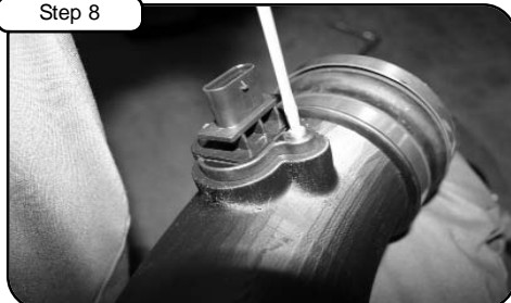
With M4 screws, gasket, and spacers provided, place MAF sensor in to new tube. (make sure gasket is between tube and sensor)
