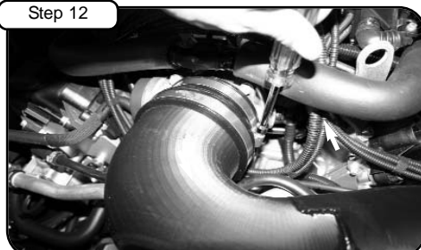
Tighten clamps using 5/16" nut driver.
