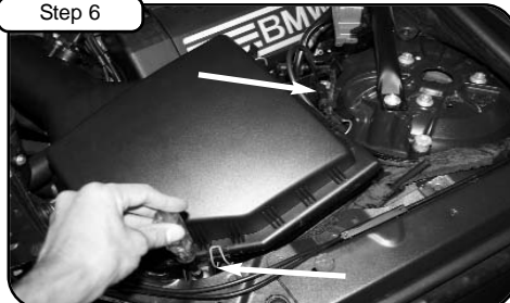
With T25 torx bit, loosen the 2 bolts that hold the OE airbox in place. Carefully remove the airbox out of vehicle.
