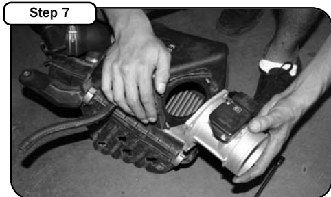
With 10mm socket or wrench carefully remove factory MAF sensor. Remove factory rubber gasket.
