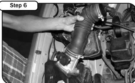
Carefully remove complete factory intake assembly out. With 10mm remove bracket from valve cover. Save 10mm bolt for future use on new housing.
