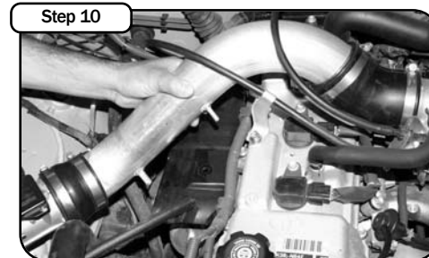
Attach couplers onto tube using the supplied clamps ( do not tighten). Place angled coupler onto throttle body side and reducer coupler on MAF side.
