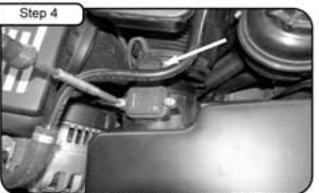
Using 1/4" nut driver, loosen factory clamp holding upper airbox. With T20 torx bit loosen the 2 bolts holding in MAF sensor. Carefully remove MAF sensor from airbox.
