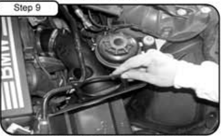
Install housing into vehicle. If your vehicle is equipped with a vacuum line see step 11 before installing tube. Place tube into coupler from step 8. With gasket provided, slide between tube and housing and wait for adapter install.
