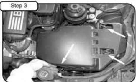
Detach the 3 Factory clips holding in upper half of OE airbox.
