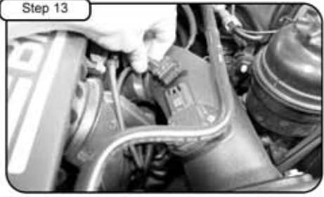
Carefully install MAF sensor into new tube. Place gasket between tube and sensor and tighten with screws provided. Connect MAF sensor harness. Tighten coupler clamps with 5/16" nut driver.
