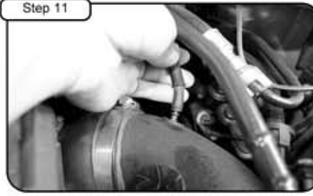
If your car is equipped with a vacuum line, drill a 0.5" hole into the tube in the location marked by the dimple. Then with the grommet, place into hole with 1/4" barbed fitting provided. Re-insert factory vacuum line.
