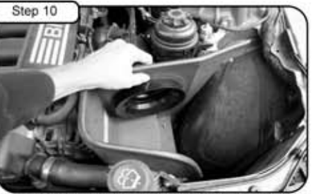
With 6" adapter, place inside of housing and with M6 screws and washers provided mount the tube to adapter. Tighten using 10mm socket or wrench. Apply trim seal to housing.
