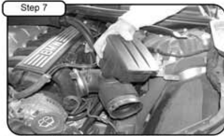
With 1/4" nut driver, loosen the clamp holding the OE intake tube @ throttle body and remove.
