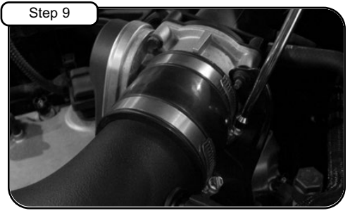
Step 9 Tighten clamps using 5/16" nut driver.
