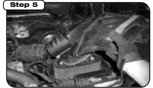
Remove top half of air box from lower half. Remove factory intake tube from factory turbo inlet elbow.
