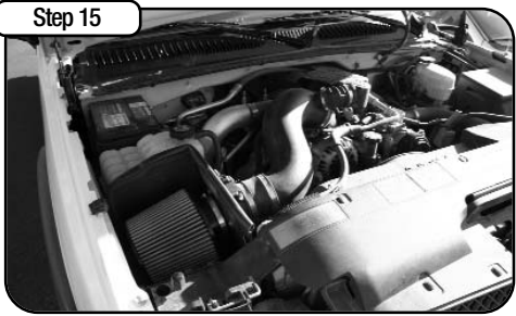
Step 15 Complete Stage 2 kit installed. Make sure all clamps are tight and all components are secure. Check and retighten connections and filter after a few hours of operation. Place the included CARB EO Sticker on or near the intake system on a smooth, clean surface. E.O. identification label is required in passing the Smog Check Inspection.
