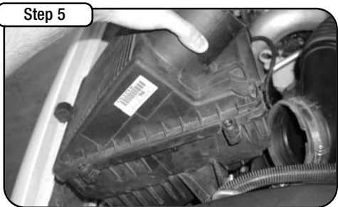
Step 5 Remove the complete stock air box from the rubber mounts. Pull up and slide sideways toward radiator.
