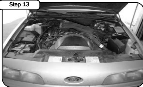
Step 13 Place enclosed CARB EO sticker on a clean/smooth surface on or near the intake system. Your installation is now complete. Make sure you tighten all clamps/nuts and check all electrical connections. Re check periodically
