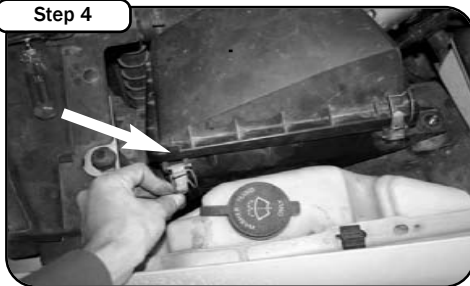
Step 4 Unclamp the 2 factory airbox clips.
