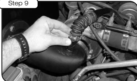
Place crankcase breather elbow onto the nipple of the plastic tube and re-tighten the coupler, be sure to not over-tighten the coupler.
