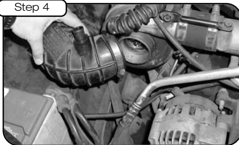
Remove factory rubber elbow at turbo.
