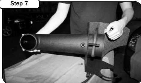
Step 7 Slide the intake duct into the housing make sure you line up the mounting holes correctly.
