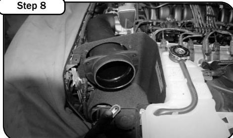
Step 8 Lower housing and tube assembly into engine bay. Make sure the tab on the back of the housing slides into the slot on the side of the radiator reservoir. Be shure to clear rubber hose near bottom of housing.
