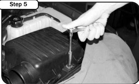
Step 5 Remove the 10mm screw securing the airbox to the vehicle. Save for re-use later.
