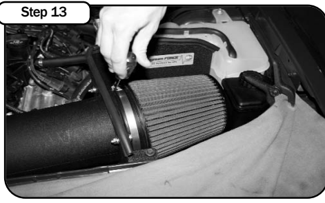
Step 13 Install and tighten your pre-oiled filter. Do not use any grease or oil.
