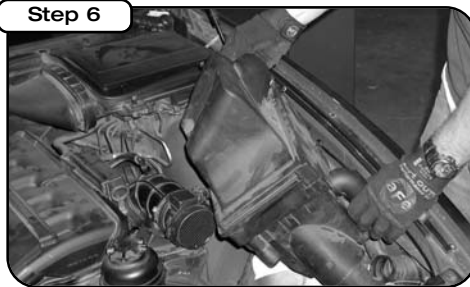
Remove OE air box from vehicle.
