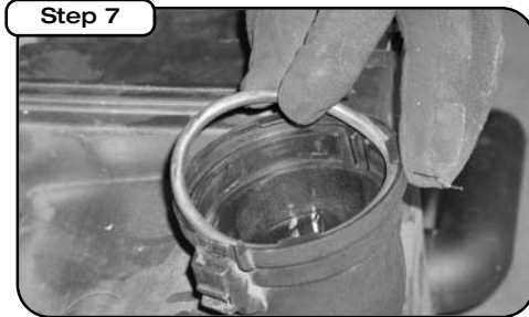
Carefully remove o-ring from stock air box.
