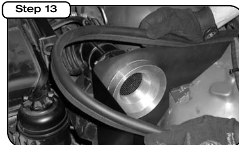
Install trim seal.
