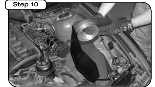
Install housing into vehicle, making sure to guide MAS into billet adapter.
