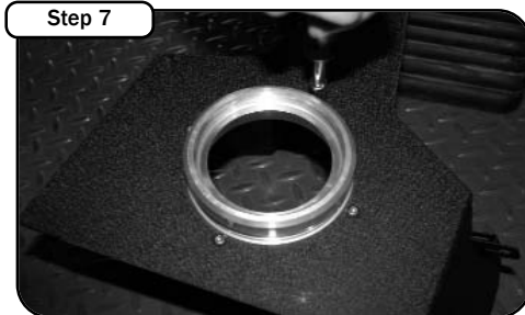
Insert the air filter adapter into the housing. Line up the four mounting holes and fasten with the supplied button head screws.
