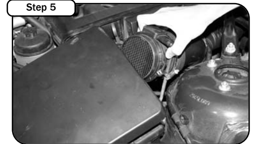
Remove MAF sensor from airbox. Make sure you do not damage the rubber gasket. Lift airbox out and remove from vehicle.
