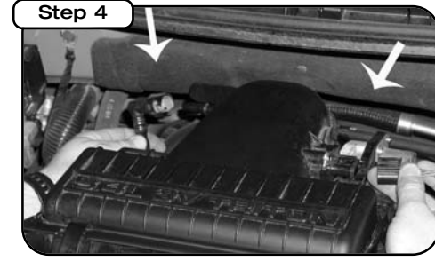
Disconnect the MAF sensor and breather tube on the sides of the airbox. Remove the 4 10mm screws holding the airbox to the intake manifold and remove intake box.
