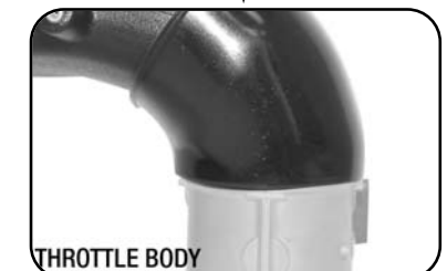
Position coupler and clamps over throttle body (3.5" x 4.0") (clamps removed for clarification). The smaller (3.5") end of the coupler goes over the throttle body. The (4") end of the coupler goes around the intake tube.
