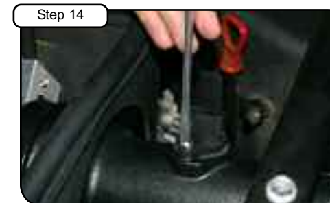
Install MAF sensor onto tube using provided gaskets and screws.
