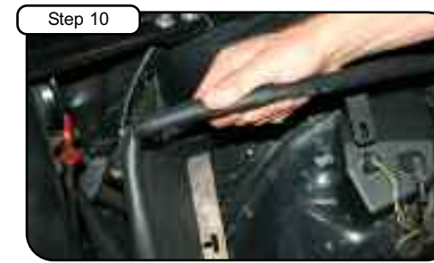
Install trim seal on housing and drop housing into vehicle. Do not tighten down housing.
