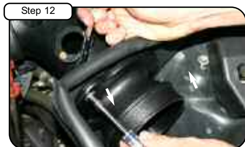
Align two holes on tube flange to holes on housing. Use provided M6 hardware to mount tube flange to housing.
