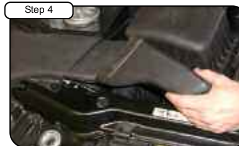
Remove front snorkel from ducting to stock airbox.
