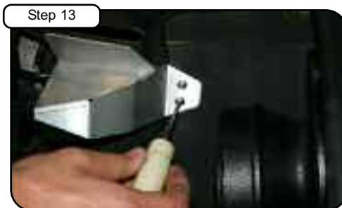
Install Flow divertor onto housing using provided button head screws.
