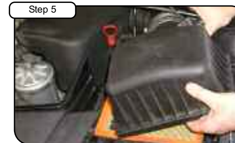
Using a standard screwdriver loosen the clamp securing intake track to factory airbox. Undo clamps securing top half of airbox and remove top half. Set aside for future removal of stock MAF sensor.
