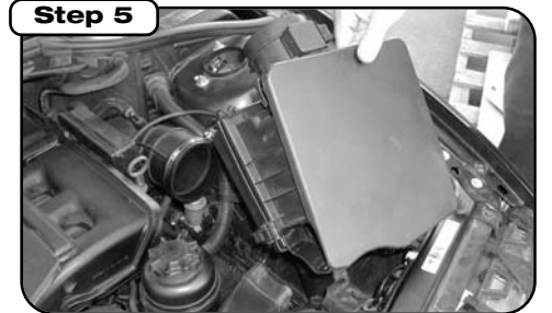
Remove OE air box from vehicle.
