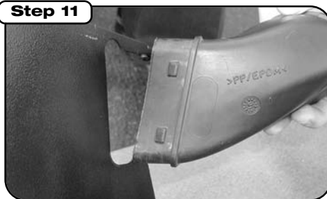
Attach stock intake snorkel onto side of shield,
