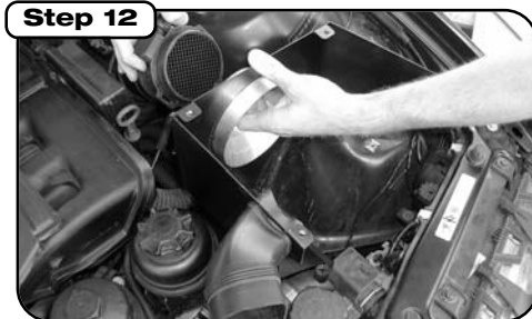
Install shield into vehicle, attach snorkel, and slip on mass flow sensor and attach spring clips.
