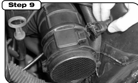
Install mass air flow sensor, tighten clamp with 1/4" nut driver and connect mass flow sensor plug.
