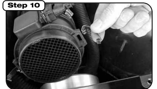
Attach supplied spring clips onto mass flow sensor insert hooked end into slotted section on mass flow sensor.
