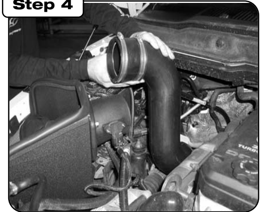
With longer (4" x 3") coupler slid onto the longer end of 419 tube, position the tube into place in the coupler on the turbo inlet. Then line up the top of tube and filter tube so you can slip the straight coupler over both tubes.
