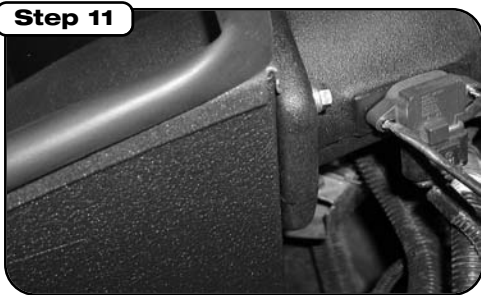
Install intake temperature sensor that was removed from the airbox onto the aFe intake tube using provided hardware and gasket, then tighten. Orientation does not matter on the temperature sensor. Re-connect factory harness to the temperature sensor.
