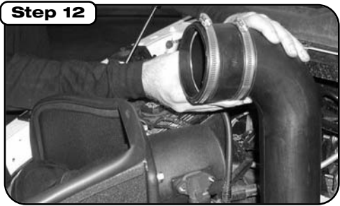
With clamps and couplers provided install high temp coupler at turbo side and 4"x3" urethane coupler at filter side, tighten using 5/16" nut driver. Install pre-oiled filter onto intake tube and tighten. Do not use any oil or grease when attaching filter. Reattach radiator overflow hose that was removed in Step 7.
