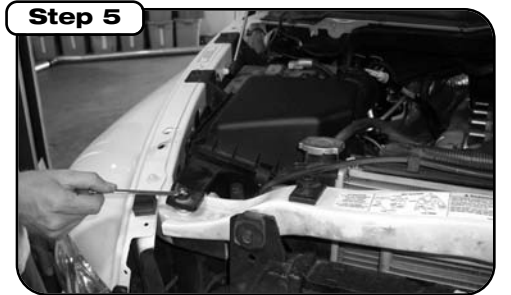
Using 10 mm wrench, remove the bolt that secures the factory airbox to the radiator bulkhead.
