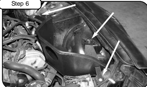
With OE screws removed from step 5, install new aFe housing to vehicle. Tighten using 10mm socket or wrench.
