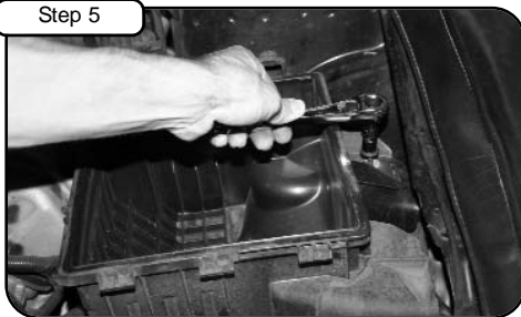
With 10mm socket or wrench loosen the 2 screws holding in OE air box. Lift up and remove OE air box out of vehicle.
