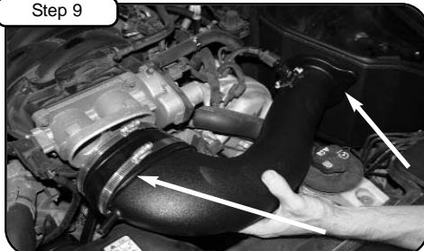
Install coupler with clamps to tube. Install tube to outside of housing and position coupler on to throttle body.
