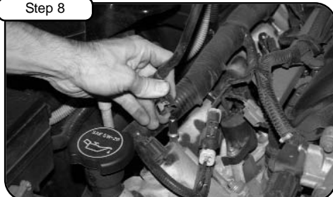
Remove factory crank case line from engine.
