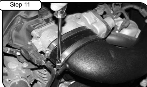
Tighten clamps with 5/16" nut driver.
