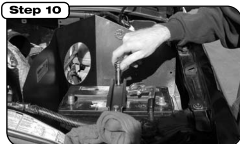
Place battery into intake housing using supplied clamp and two 8" long hex head bolts and locking washers. (DO NOT OVER TIGHTEN).
