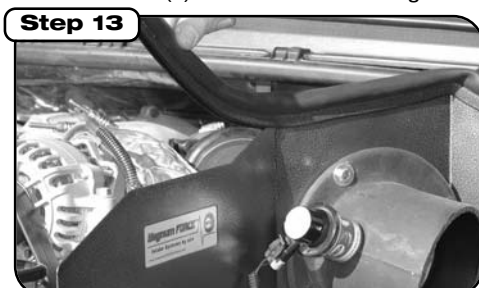
Install trim seal on housing.
