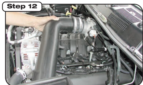
Thread filter end of housing through opening in filter housing first, then slip coupler over throttle body. Tighten clamps at throttle body.
