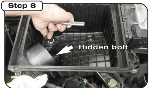
Remove four bolts from lower half of air box. Note: There's a bolt hidden underneath airbox inlet tube. You must use an open end wrench or adjustable wrench to remove.
