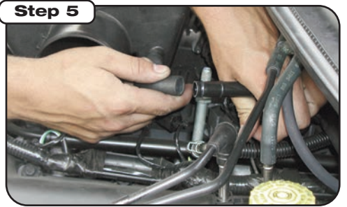
Remove vent hose at tubing coupler.
