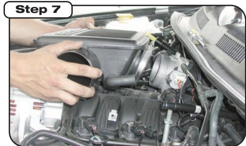
Loosen clamp at throttle body and remove resonator box from throttle body.
