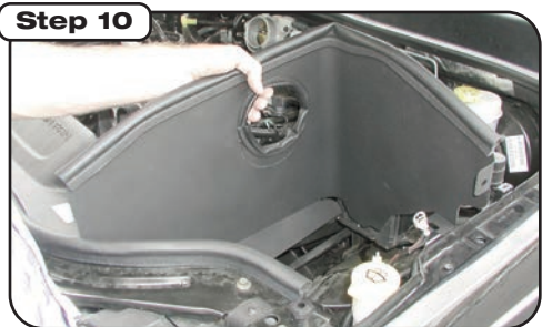
Before installing housing, apply large trim seal to top of housing and small trim seal to tube inlet. Install filter housing using supplied hardware on lower mounts.
