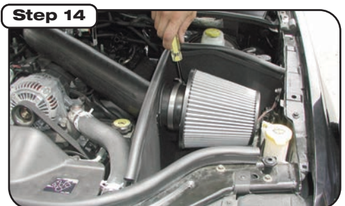
Install filter to intake tube and tighten clamp.
