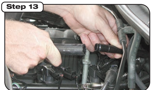
Connect supplied vent hose to nipple at intake tube and at breather vent tube. Note: no clamps are required.
