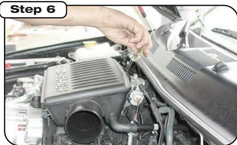
Loosen clamp at throttle body and remove resonator box.
