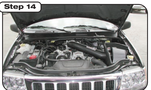
Place enclosed CARB EO sticker on a clean/smooth surface on or near the intake system. EO identification label is required in passing Smog Check inspection. Make sure all hoses and clamps are tight and that all electrical components (if applicable) are secure. Check and retighten connections and filter after a few hours of operation.
