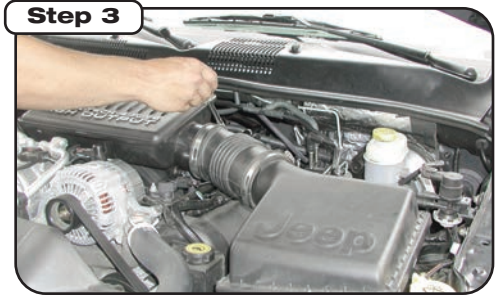
Loosen clamp at air resonator box and remove top half of filter box.
